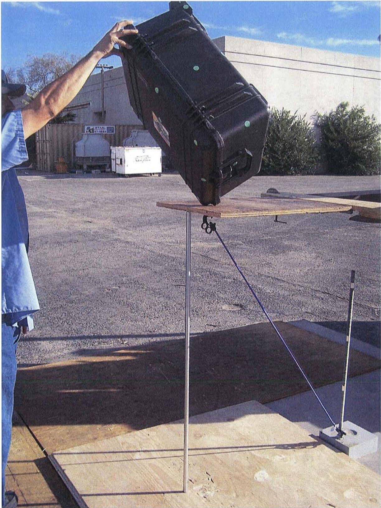
Photograph 13 Transit Drop Test – Typical Corner Drop
