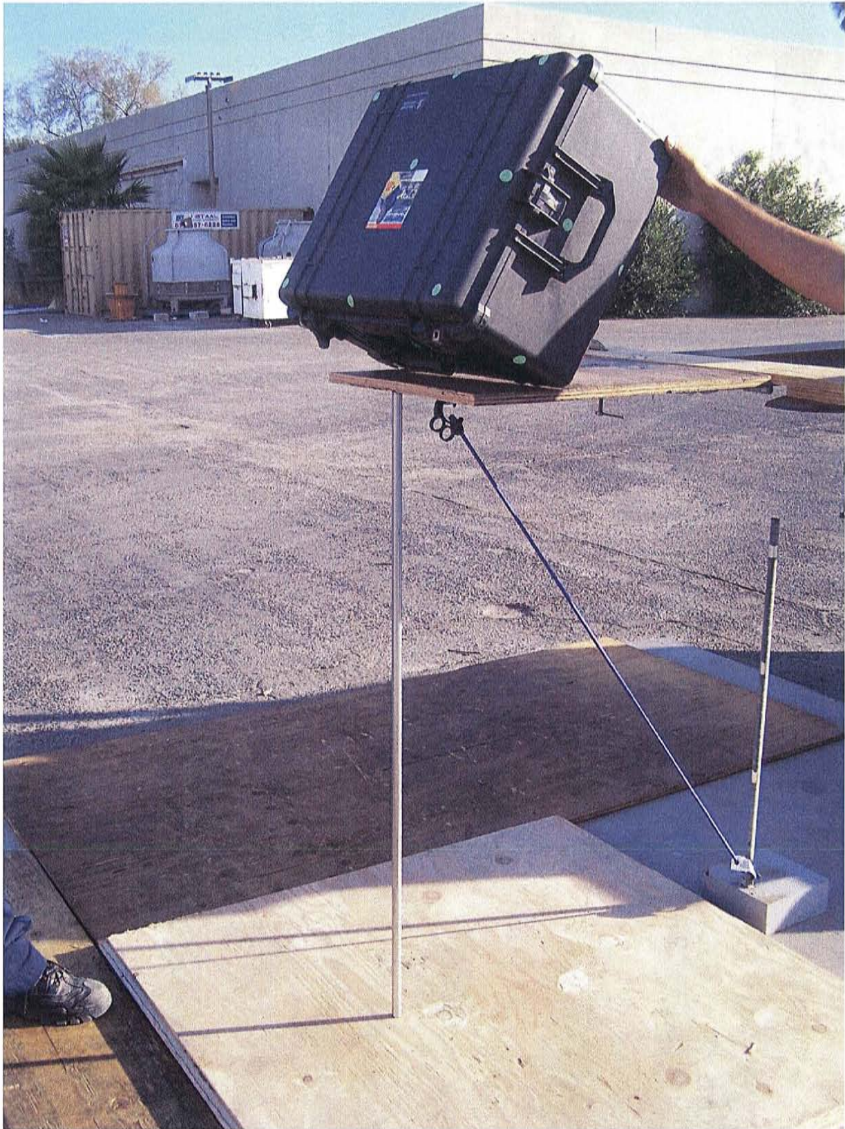
Photograph 12 Transit Drop Test – Typical Edge Drop
