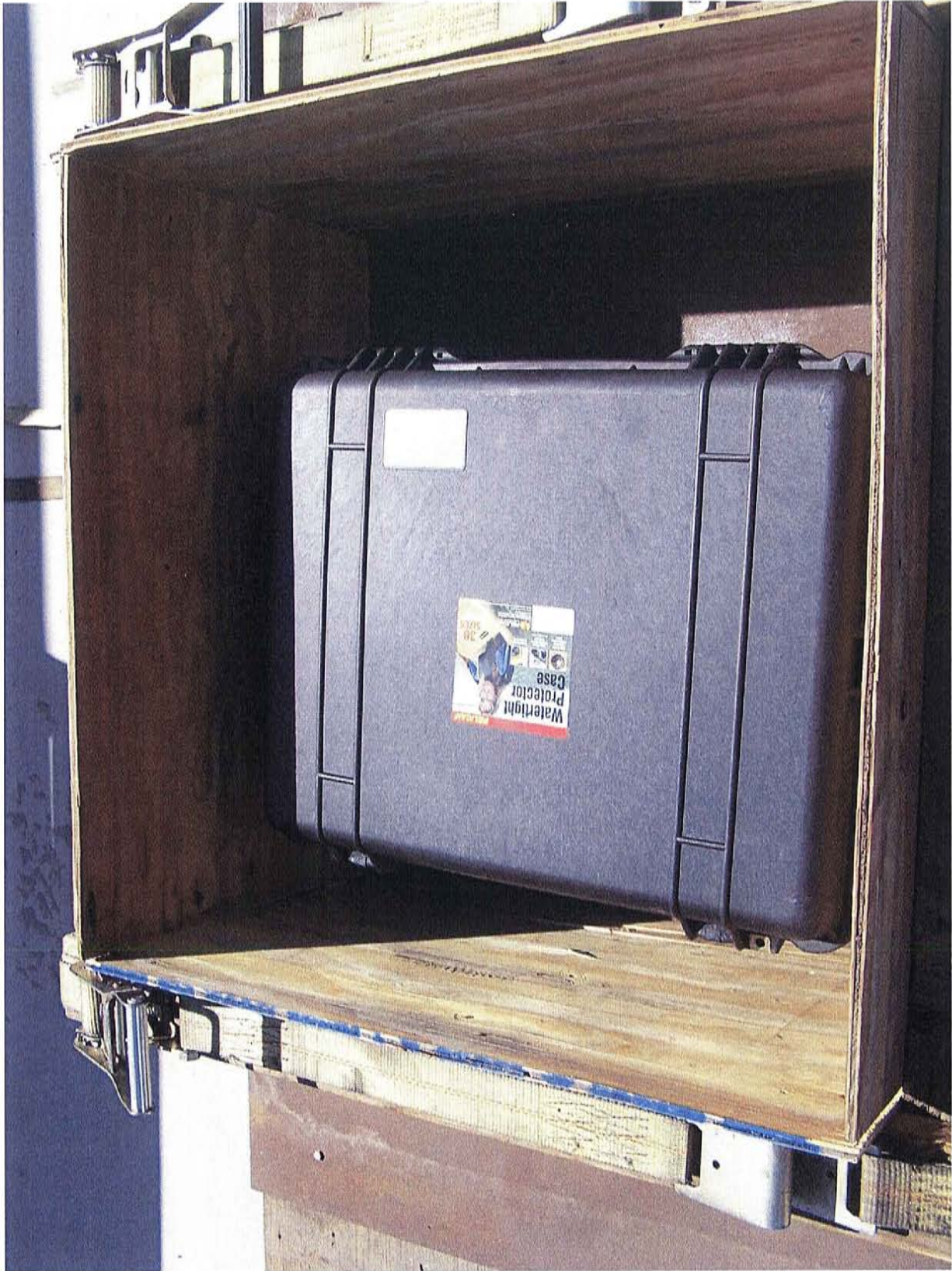
Photograph 6 Loose Cargo Transportation Test – Transverse Direction
