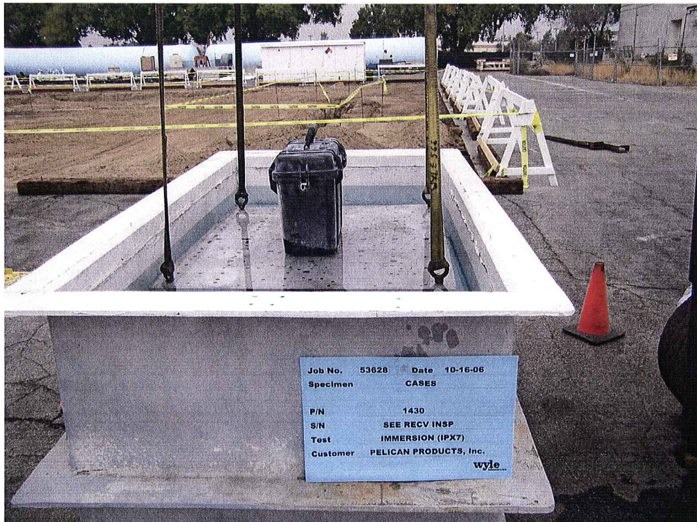
Photograph 4 Immersion Test Setup
